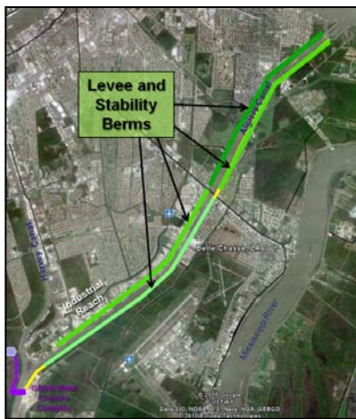
All four levee lift and stability contracts are complete. Levees elevation is 8.2 ft.
